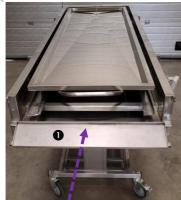
Integration of the stretcher inside the tank, with a tilting panel at one end ① to close the tank and the air extraction manifold ② at the other end.
