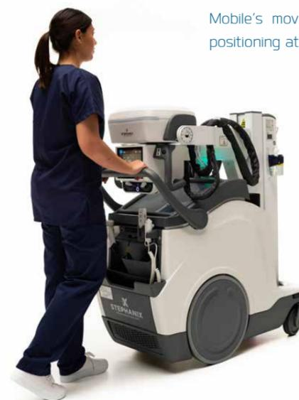
Movix DReamy rear diameter load wheels, as well as front steering wheels featuring shock absorbing springs help to cross obstacles such as elevator threshold.
