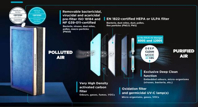
All our filter units are medical-grade certified and are manufactured in France. They are individually inspected and tested so as to guarantee optimal efficacy.
